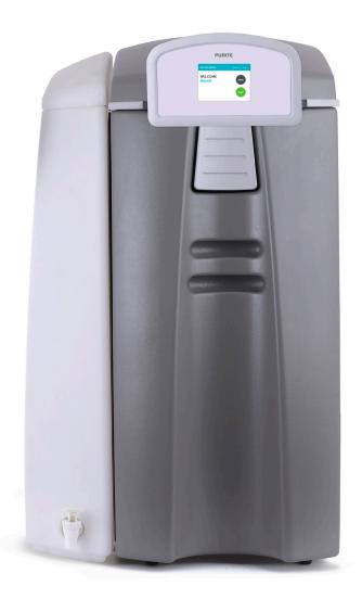
The Purite Analyst is a compact unit ideal for laboratory use, delivering a steady supply of >  $1M\Omega$ .cm pure water for laboratory tasks using carbon pre-treatment, reverse osmosis and deionisation. Typical applications include glassware rinsing, buffers and stains, reagent make-up, and media preparation.
