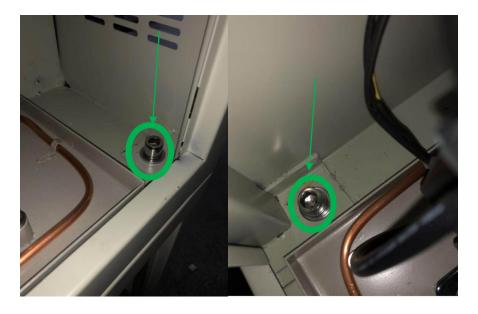
4. Use Allen key to unscrew the inner hexagon bolts to perform the stacking or unstacking operation.
