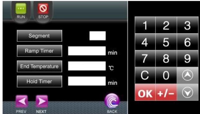
This new incubator can operate according to stored program to meet various requirements of professional experiments. Under programmable control mode, it is possible to program up to 9 different segments, each with their own Ramp Time, Ramp End Temperature, Hold Time and Speed. At the end of the settings, you are also required to set the Hold Deviation and Cycle Times.
