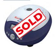
The SciSpin Micro Centrifuge offers very high performance for such a small microfuge. This powerful, high speed microfuge is compact and light enough to be portable and is ideal in any laboratory where bench space is at a premium.
