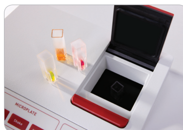
Cuvette port for standard and micro cuvettes
