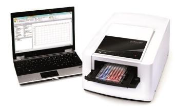
Novel LED technology provides a worry-free operation without compromising on measurement performance. LEDs rarely require replacement unlike traditional halogen lamps.
