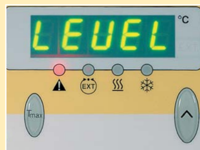
Alarm message for malfunction
