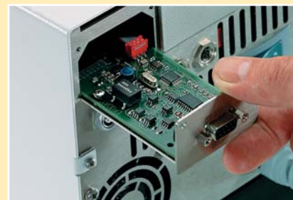
Easy replacement of interface modules
