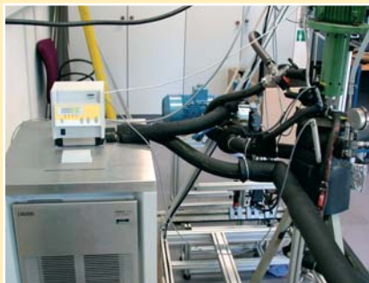
Cooling of reactors for examination of the formation of gas hydrates
